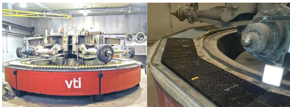
Figure 4. The CRS setup in VTI and illustrations of fixing the FIBRA plates to the track [5]
