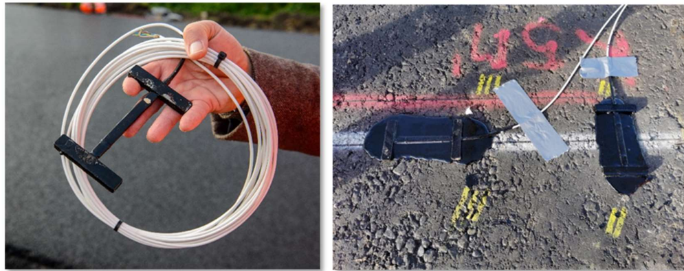
Fig. 3 Schematic of strain gauge (left) and its installation at the top of the bottom layer (right).
